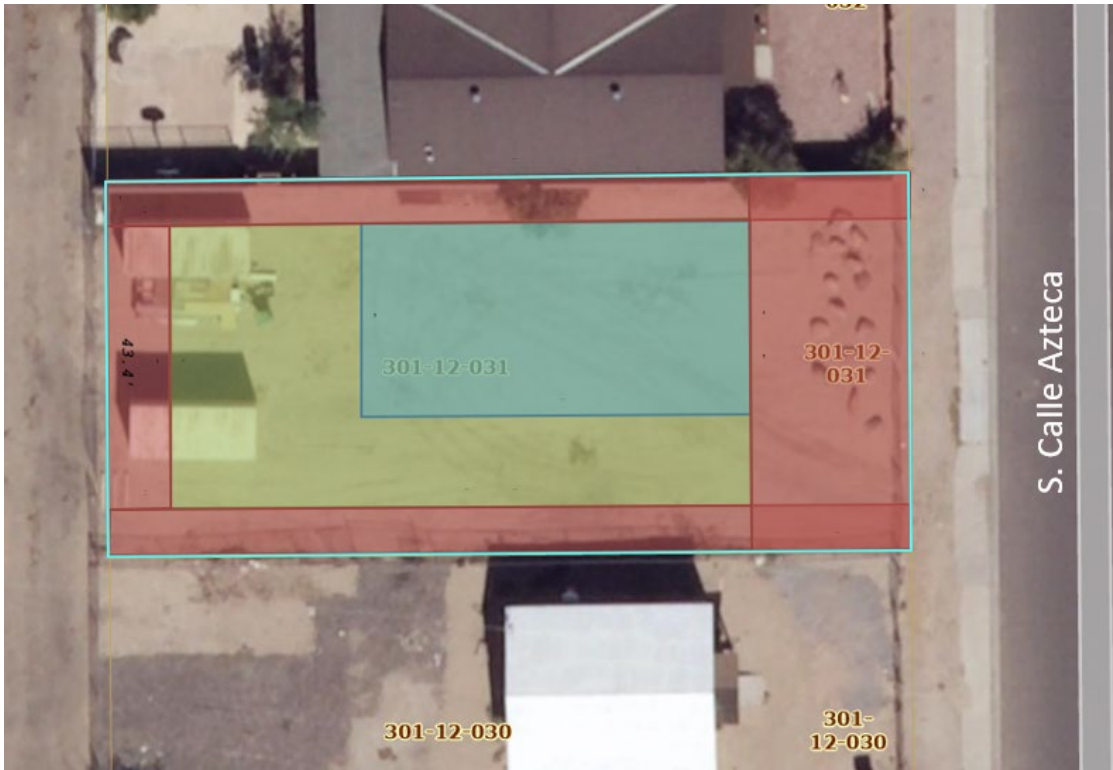
Exhibit B – Manufactured Home Building Footprint & Setbacks
